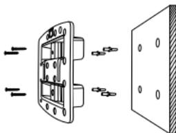
1. Put the mounting bracket to the wall with screws;
