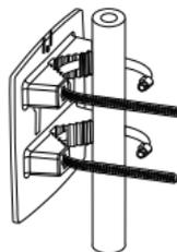
2. The mounting bracket is locked on the pole by a metal hoop;
