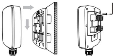
2. Put the device on the mounting bracket and push it down until it connect into position and lock the fixing screw between the device and the mounting bracket.
