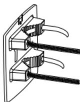
1. Insert the metal hoop into the mounting bracket;
