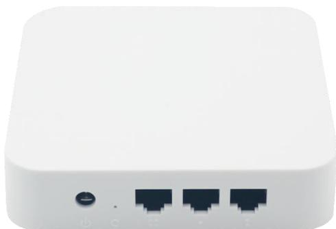
GAP56B, a gateway AP with multiple functions dedicated for small-and-medium stores, is from ABLOOMY Technologies Inc. (ABLOOMY)' s self-led research and development. Taking wired and wireless network, VSM is equipped with an uplink port connecting Internet, 2\* Ethernet ports and 802.11b/g/n port which supports 300Mbps transmission rate. GAP56B support both gateway function and 802.11b/g/n client accessing.
